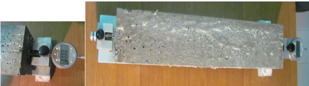
Test ritiro UNI 11307 – Misure 100x100x500 mm
